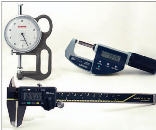
Above: These three measuring instruments offer different levels of precision as shown on the scale of each one. The pearl gauge can be read to  $\pm 0.05$  mm, the slide micrometer to  $\pm 0.01$  mm (or 0.0003 inches) and the digital screw micrometer is precise to  $\pm 0.001$  mm.
